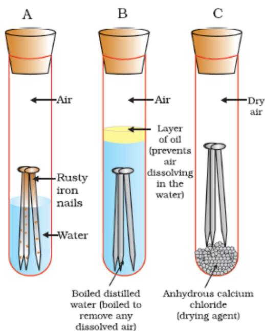
You will observe that iron nails rust in test tube A, but they do not rust in test tubes B and C. In the test tube A, the nails are exposed to both air and water. In the test tube B, the nails are exposed to only water, and the nails in test tube C are exposed to dry air. What does this tell us about the conditions under which iron particles rust?
